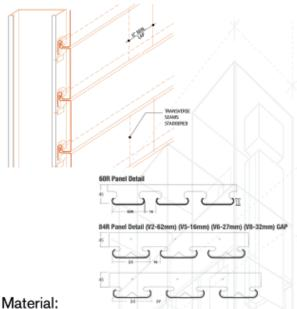
0.50mm galvanized steel provides a budgetfriendly solution. 0.55mm Alu Zinc delivers superior protection against corrosion, ideal for harsh environments. Or lightweight 0.65mm aluminum TCT.
